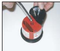
Note: If necessary, prime the MEMOLUB<sup>®</sup> HPS with a hand grease gun.
