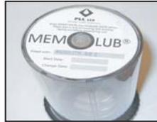
2. Remove the paper, disk-shaped label from the replacement cartridge and fill in the "Start Date" and "Change Date".
