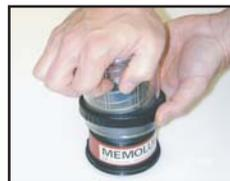
5. Place the clear housing assembly over the lubricant cartridge and red housing.
