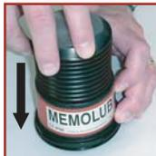
4. While holding the cartridge and red housing together, flip the assembly over and hold the cartridge in place.
