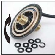
1. Program the volume of lubricant output by inserting the stroke-limiting washers.
