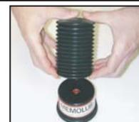
4. Place the cartridge on the inlet of the red housing.
