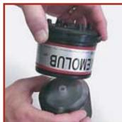
3. Hold the cartridge with the outlet facing up. Carefully remove the cartridge plug. Turn the red housing over and gently place it on the outlet of the cartridge.
