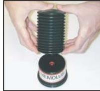
4b. Place the cartridge on the inlet of the red housing.
