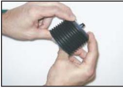
4a. Carefully squeeze air out of the cartridge until grease begins to emerge from the outlet.
