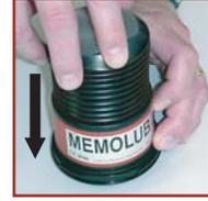
5b. While holding the cartridge and red housing together, flip the assembly over and hold the cartridge in place.
