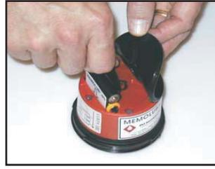
2. Lift back the black rubber seal and insert the battery pack.
