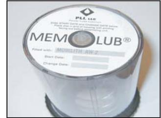
3. Remove the paper, disk-shaped label from the replacement cartridge and fill in the "Start Date" and "Change Date".
