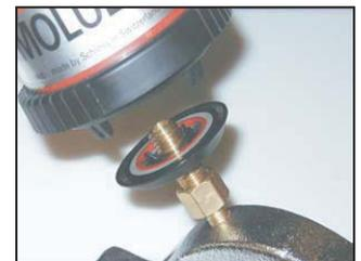
9. Screw the MEMOLUB<sup>®</sup> HPS lubricator onto the MEMO.
