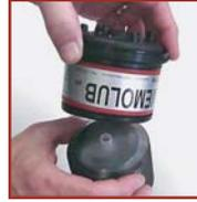
5a. Hold the cartridge with the outlet facing up. Carefully remove the cartridge plug. Turn the red housing over and gently place it on the outlet of the cartridge.
