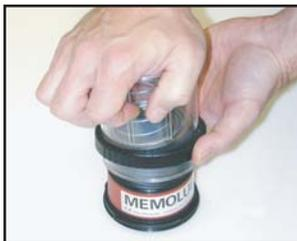
6. Place the clear housing assembly over the lubricant cartridge and red housing.
